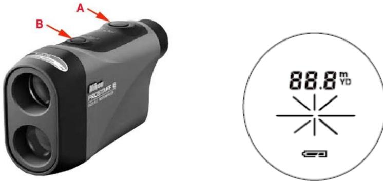
To take a measurement press the Power button **A** and the LCD illuminates, align the reticle on the target and press and hold the Power button again until the display appears as it does in the picture, right side above. To obtain the best results try to select bright coloured targets with large, shiny, highly reflective surfaces.
